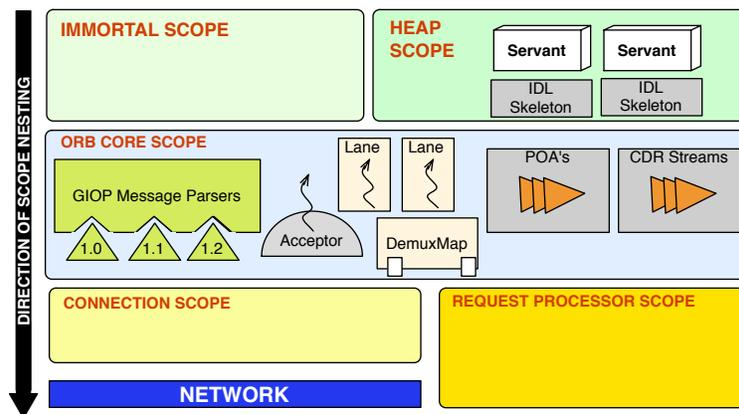
Figure 5: Scoped Zen Server Scoped Memory Architecture.
