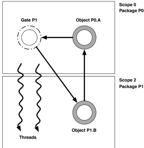
Figure 2: *Programming Model*. Each runtime scope has a corresponding Java package. Objects defined in a package are always allocated in the corresponding scope with the exception of the scope's Gate which is allocated in the parent scope. All legal reference patterns are shown.
