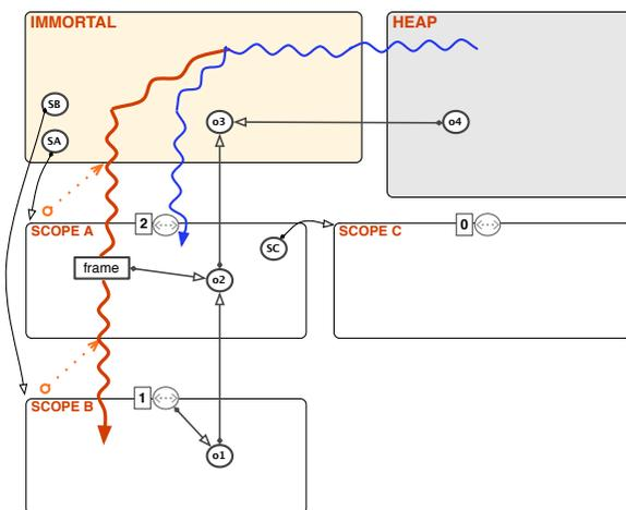
1. Scoped memory areas (A, B, and C) are represented by special meta-objects, instances of `ScopedMemory`, allocated in another scope (SA, SB, and SC).
